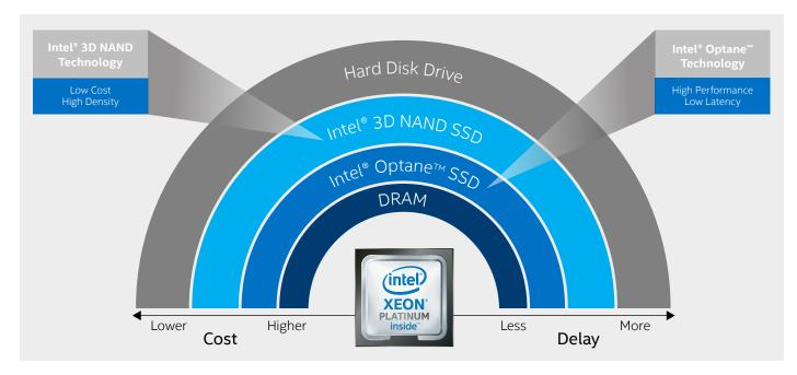
Figure 1. Intel<sup>®</sup> Optane<sup>™</sup> technology introduces a new layer to the storage infrastructure
